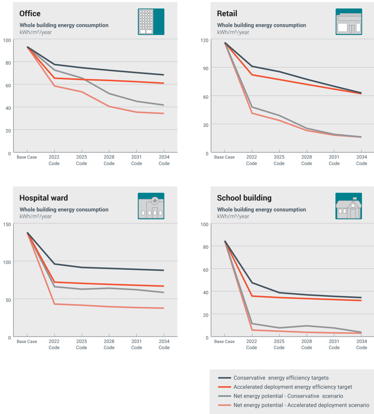
FIGURE A1: Summary of energy efficiency targets and net energy potential, averaged across the four modelled climate zones ... continued
