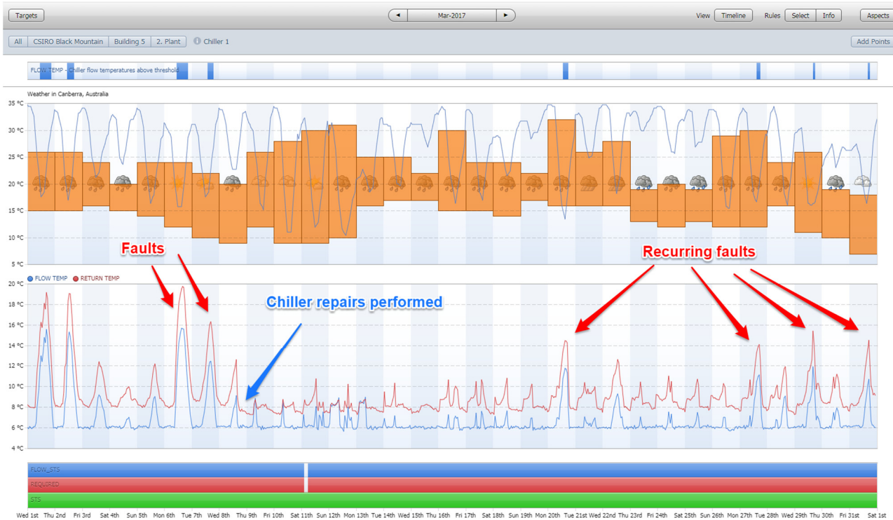
Figure 28. C&E Analytics (CSIRO Building 5) - Issue: Chiller faults
