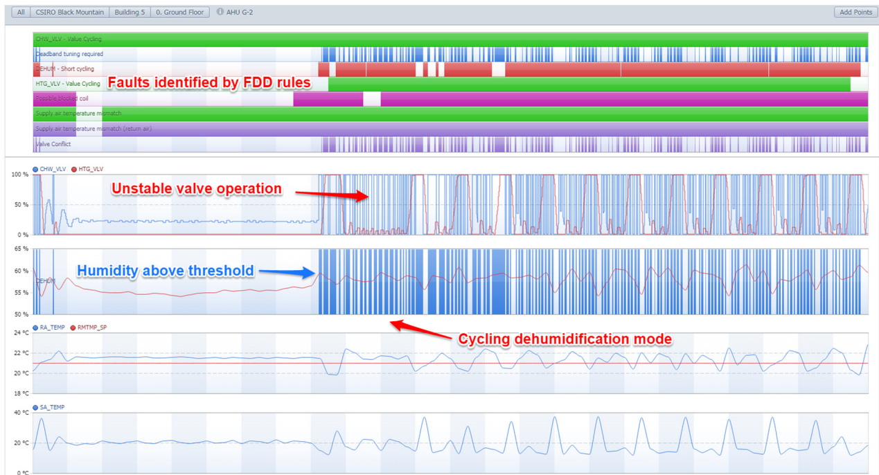
Figure 29. C&E Analytics (CSIRO Building 5) - Issue: AHU G-2 short cycling dehumidification mode
