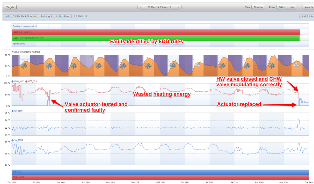
Figure 27. C&E Analytics (CSIRO Building 5) - Issue: AHU 1-4 leaking chilled water valve
