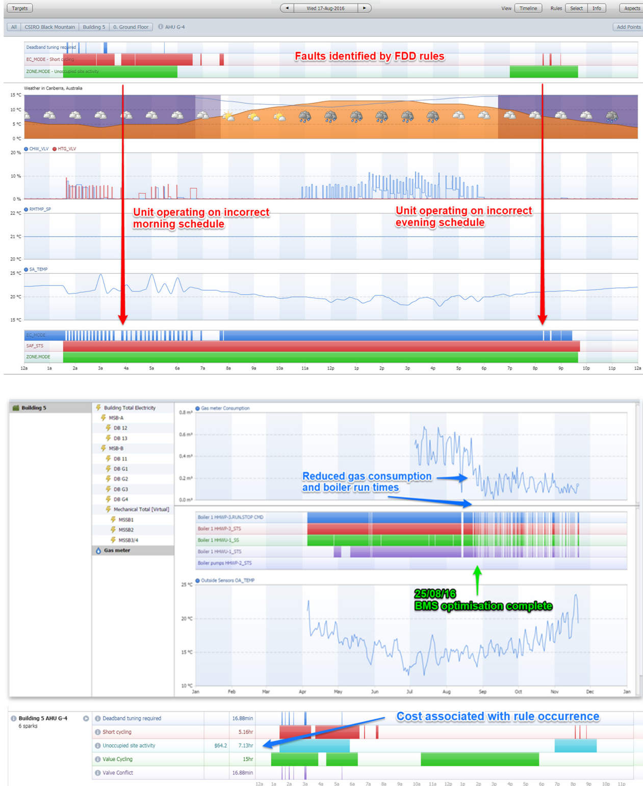
Figure 30. C&E Analytics (CSIRO Building 5) - Issue: HHW tuning – reduced demand
