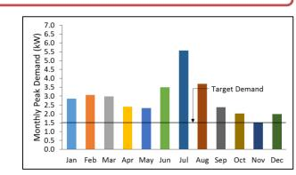
Figure 4: Monthly Peak Demands Using CS4 with 2.5 kWp PV and 1 kWh Battery.
