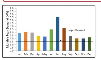
Figure 3: Monthly Peak Demand Using CS4 without PV and with 1 kWh battery.
